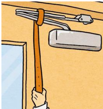
Secure a belt, rope, or cable around the top of the door hinge.
